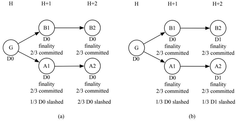
Fig. 17: Revert Two Blocks by Short-range Attack
