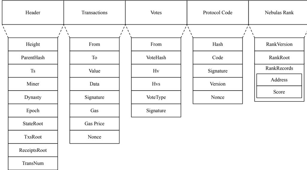
Fig. 9: Block Structure
